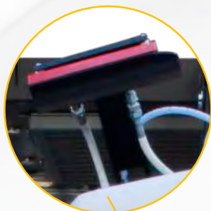
Dispositivo pressa-spalle teflonato Teflon-coated shoulder pressing device
